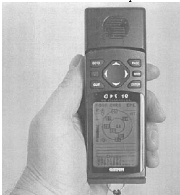
Figure 2.11 A Garmin GPS-12 , typical hand-held GPS instrument. It can locate you to within a few metres on the ground and assist you in following a specific route. It cannot be used in forest because it requires a clear view of several satellites. It also does not function well in icy conditions.
