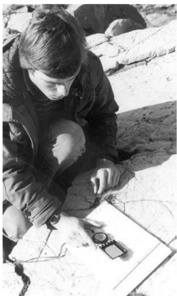
Figure 5.1 Measuring strike by the contact method, Figure 5.2 Using a 'Dollar' type clinometer to measure dip
