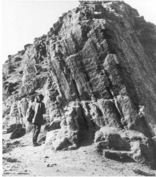
Figure 5.3 Measuring the strike of a veinlet on a rough horizontal surface by Method 2, Figure 5.4 An ideal exposure for the end-on measurement of dip
