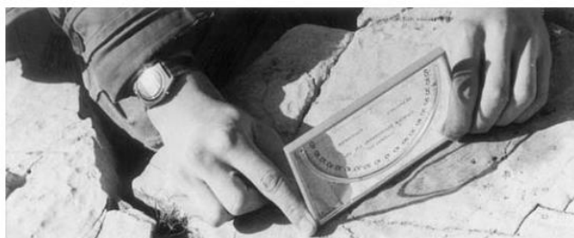
Figure 5.1 Measuring strike by the contact method, Figure 5.2 Using a 'Dollar' type clinometer to measure dip
