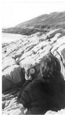
Figure 5.5 Measuring the strike of an uneven surface with a prismatic compass (Method 3)
