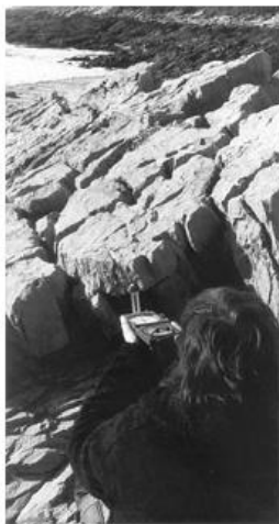
Figure 5.5 Measuring the strike of an uneven surface with a prismatic compass (Method 3)
