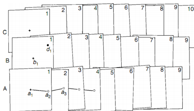
Figure 2.7 A block of three runs of aerial photographs, A, B and C. Photographs in each run overlap each other by 60% so that the position on the ground of the principal point (a) of photograph A-1 can also be found on photograph A-2. Similarly the pp on photo A-2 is found on both photos A-1 and A-3. Adjacent runs overlap by about 30% so that a feature d seen on photo B-1, can not only be found on photo B-2 and B-3, but also on photos C-1, C-2 and C-3 of the adjacent run
